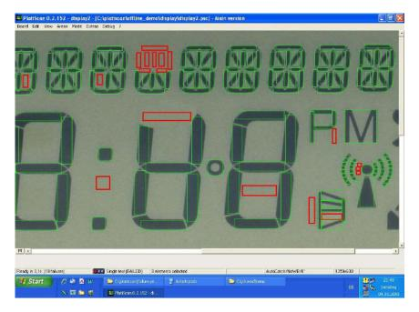
The system consists of a photo-camera, to be positioned above the Display, a PC Controller and the **PlatiScan VI**-Software. Then an image is taken via remote control and an RGB analysis is done on the PC. The detected failures can be reported as text or graphically displayed.
