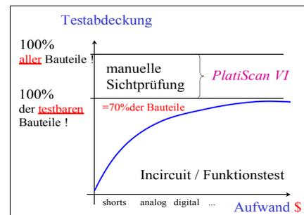
The goal is either to decrease the gap of untested devices left by the electrical In-Circuit-Test (Incircuit- and Functional Test usually cover only about 70% of all components). Or, to check all components extracted from CAD-data.
